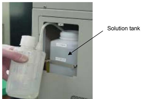
Fig.4 Solution tank
