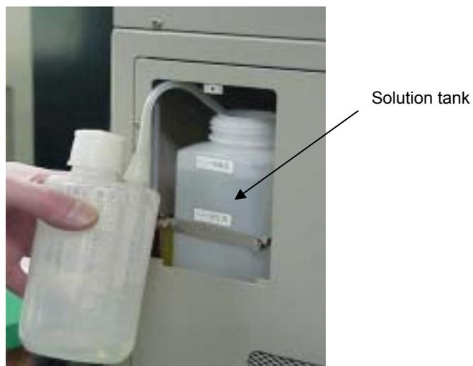
Fig.14 Solution tank
